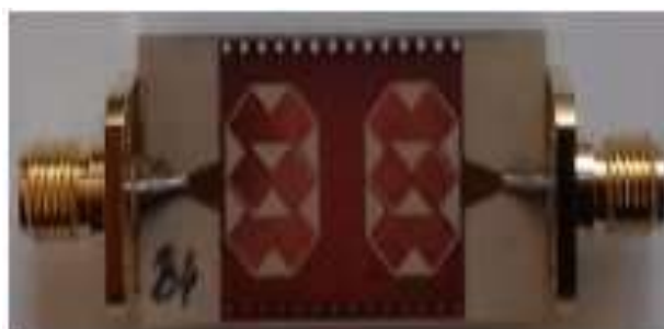
Figure 18. Photograph of the fabricated two-stage SIW bandpass filters using proposed CSRR with nested configuration.
