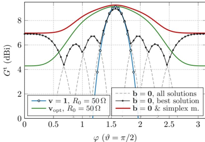
Uniform array of four metallic dipoles,  $d = \lambda/2$ .
