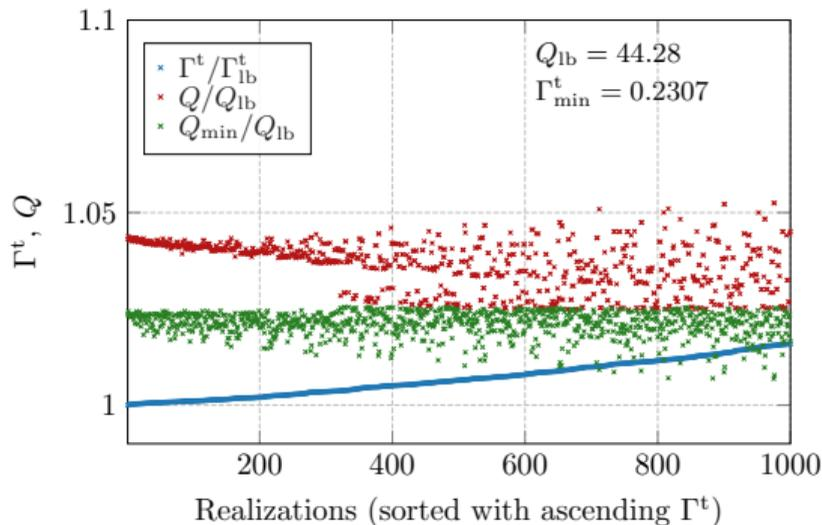
Comparison of TARC and Q factor for fed metallic rims. Excitation found via QCQP, placement via combinatorial optimization.
