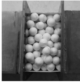
Fig. 5. The amorphous metamaterial in the partly disassembled measurement setup.
