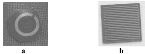
Fig. 1. The fabricated BC-SRR (a), and the fabricated planar NEP resonator [12] (b).
