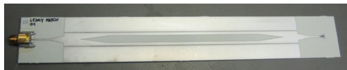
Fig. 1. Fabricated antenna radiating from a slot in the SIW top wall [4].
