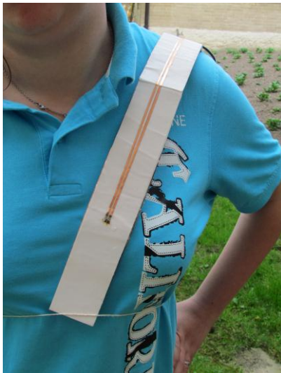
Figure 5. Photograph of manufactured coupled patches antenna placed over shoulder during tests.
