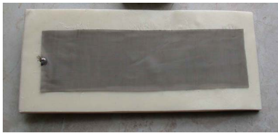
Fig. 2 Transponder patch antenna with chip, a) schematic view, b) photograph of designed prototype
