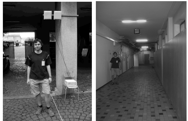
a) b) Fig. 4. Photograph of test configurations: a) a person with a chest-fixed TAG in an open area, b) a person with a chest-fixed TAG in a 4 m wide corridor
